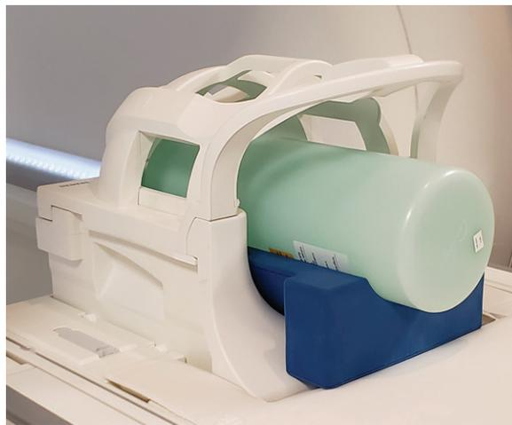
**Figure 26.** Photograph shows testing of an RF coil using the dedicated phantom and phantom holder specified by the MRI system manufacturer.
