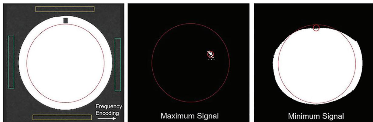
According to the ACR approach, mean SNR = mean signal in phantom/background noise. “Mean signal in phantom” is the signal magnitude (large red circle) measured from a region-of-interest that covers most of the cross-sectional area (> 75%) of the phantom.
