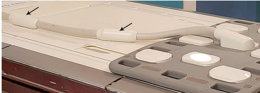
**Figure 13.** Photograph shows cable traps (arrows) along the cable of an RF coil.
