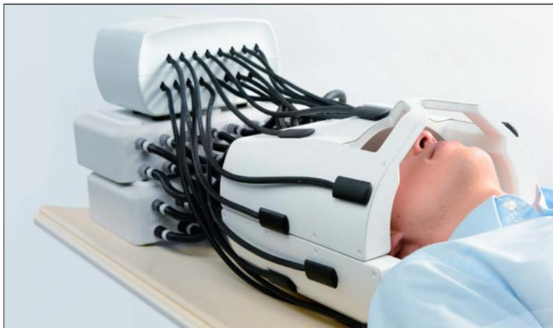
**Figure 1.22** A photograph of a commercial field-monitoring system using a series of microcoils (encased in black plastic), tuned to the fluorine resonance, with a fluorinated sample inside. By continuous measurement of the phase of the fluorine MR signal, spatial and temporal variations in the magnetic field can be measured and corrected either in real-time or in signal post-processing.
