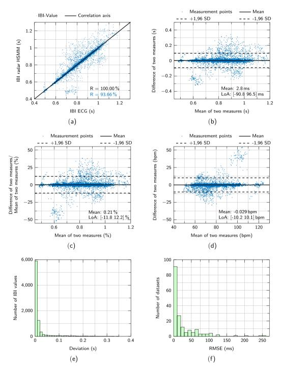
**Fig. 4** Performance comparison between radar and ECG. Scatter diagram (**a**) and Bland-Altman (**b**) plot of all IBI values. (**c**) shows the same Bland-Altman plot but with the differences plotted as percentage of the mean values. (**d**) shows the Bland-Altman plot with bpm values. (**e**) Histogram showing the deviation of all IBI values from their reference. (**f**) Number of datasets that have a certain RMSE.
