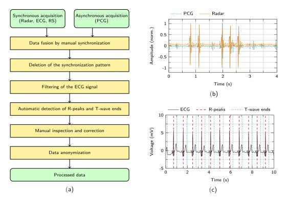
**Fig. 3** Synchronisation and reference labeling. (**a**) A flowchart showing the signal acquisition, synchronisation and ECG reference labeling process. (**b**) The tapping pattern used at the beginning of every measurement that is used to synchronise radar and PCG signal. (**c**) An exemplary reference labeling of an ECG signal showing the R-peaks and the T-wave ends<sup>17</sup>.
