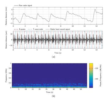
**Fig.** 7 Effects of speech on the measurement. (**a**) A cutout of a raw distance signal and the corresponding radar heart sound signal of test subject 3 while reading a text. (**b**) Short-Time Fourier Transform of the radar signal in (**a**) bandpass-filtered with a passband of 16 Hz and 1000 Hz.
